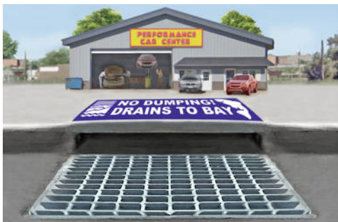
Storm Drain: An outdoor drain that flows directly to creeks and the Bay.
