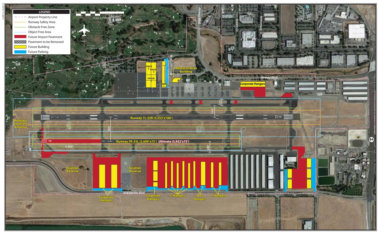
the width at 100 feet. The design aircraft is planned to remain B-II-3, which is represented by a combination of the Falcon 900B and Cessna Citation X (750) business jets. The runway design code (RDC) will remain B-II-2400 and the runway reference code (RRC) will remain at B-I-2400/B-II-4000. Under ideal conditions, the RDC and the RRC would be the same; however, the existing runway system predates the FAA design standards.
