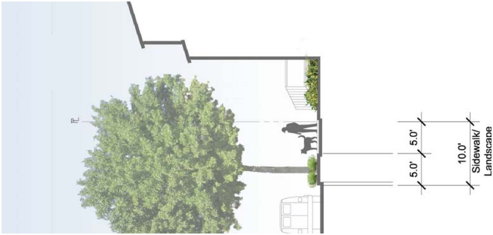
Bennett Drive and Arroyo Vista Road Sidewalk Condition (Section C)
