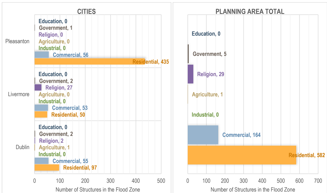
Figure 11-8. Structures in the 1% Annual Chance Flood Zone, by Jurisdiction and Occupancy Class
