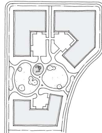
Buildings should define street edge and provide enclosure for semi-private community open space.
