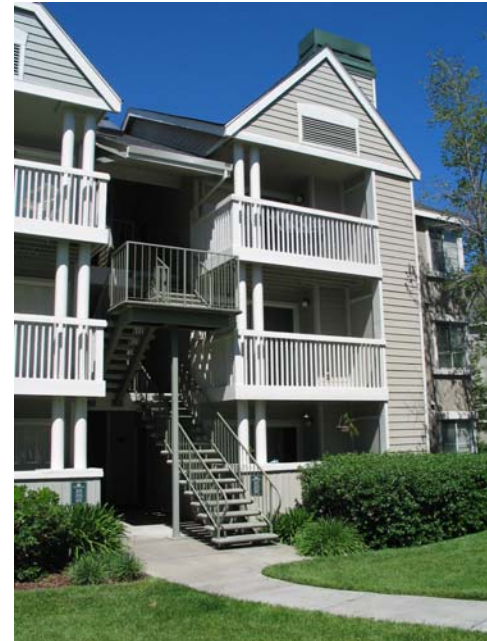
Balconies should be of sufficient size to accommodate at least two chairs and a table.
