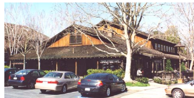
Upper floor setback and varied roof massing break down large building volume.
